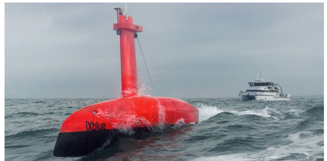
NOAA's Office of Coast Survey and the University of New Hampshire's Center for Coastal and Ocean Mapping/Joint Hydrographic Center are working with iXblue to evaluate the "DriX" USV as a force multiplier by working in tandem with research ships to increase rates of ocean-bottom mapping. Photo credit: iXBlue.
