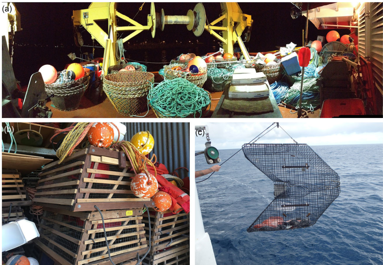
Figure 3 Three examples of traps used by scientists to survey fish or decapod crustaceans. (a) Annual snow crab ( Chionoecetes opilio ) survey using baited traps to estimate relative abundance and monitor animal health in Notre Dame Bay, Newfoundland, Canada, aboard the Canadian Coast Guard Ship Vladykov (photo credit: Darrell Mullowney). (b) Mesh-enclosed wooden pots used to survey western rock lobster ( Panulirus cygnus ) populations in Western Australia (photo credit: Ash Miller). (c) Chevron or arrowhead traps used to monitor reef-associated fish species by the Southeast Reef Fish Survey along the southeast United States Atlantic coast (photo credit: NOAA).
