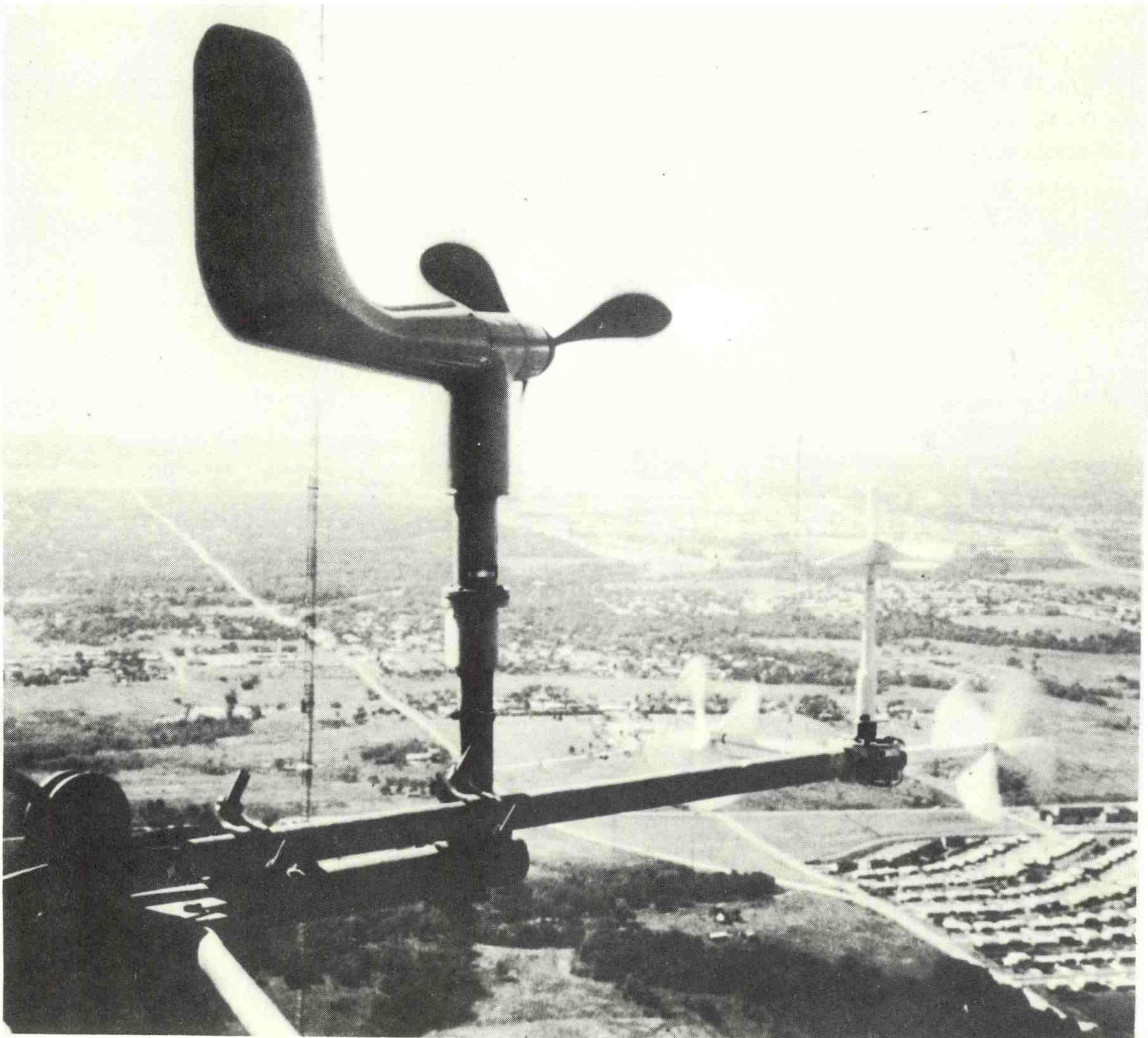
Figure 8. The orthogonal propeller anemometer in the extended position. At this time the propeller anemometer and the aerovane were being compared, normally the aerovane was removed to avoid interference.
