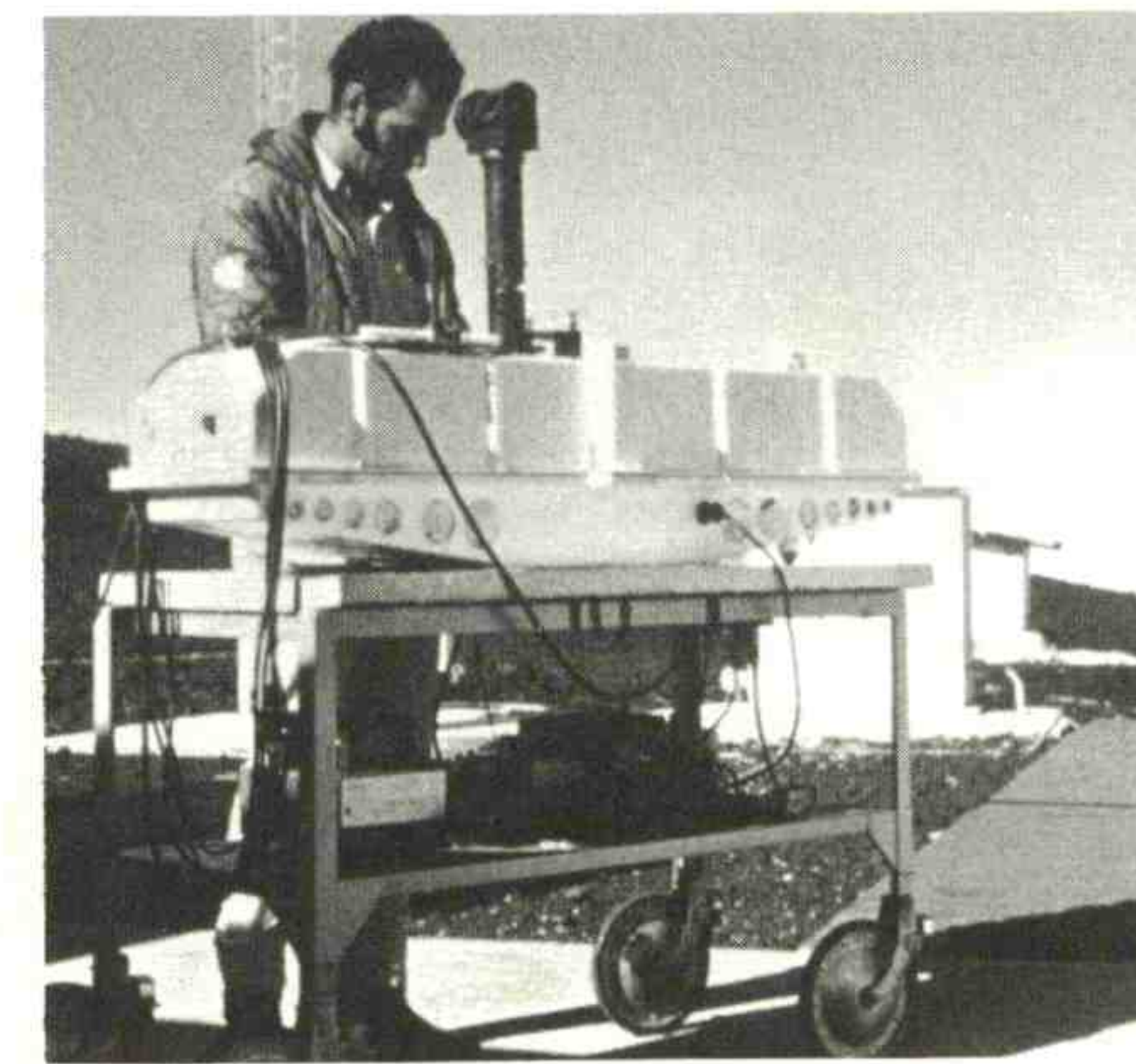
Bernard Mendonca measuring ozone with a Dobson spectrophotometer, March 1972.
