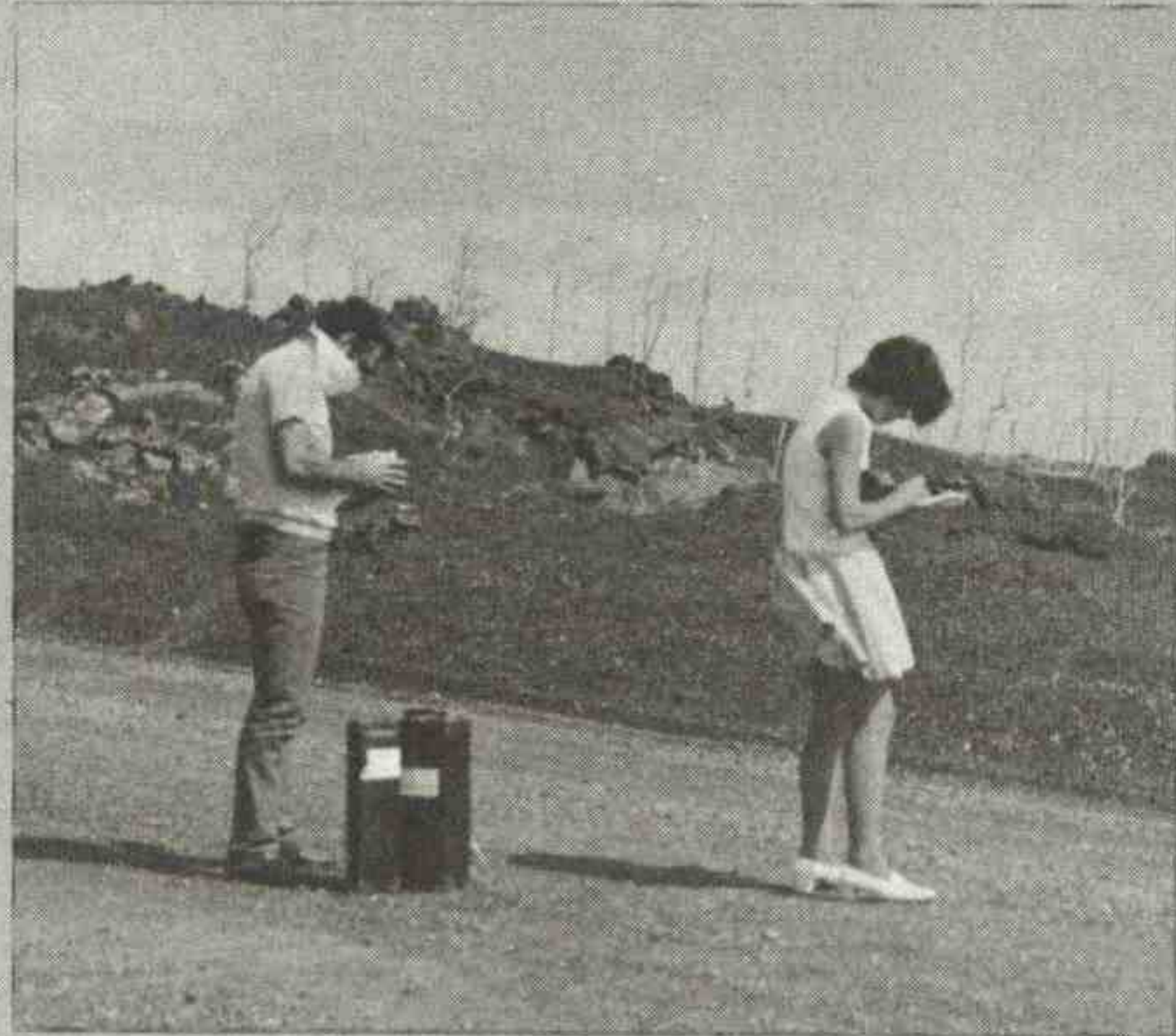
Measuring condensation nuclei with Gardner counters at Kilauea volcano during an eruption in 1969 (Bernard Mendonca and Janice Sias).
