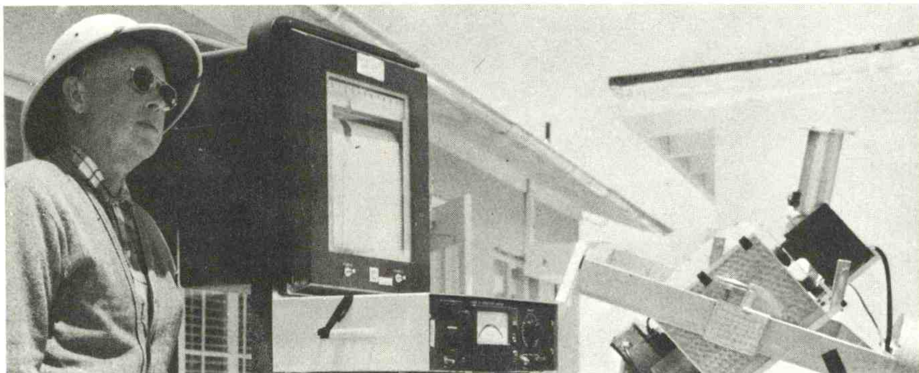
Ralph Stair making solar radiation measurements with a scanning photometer, August 29, 1966.
