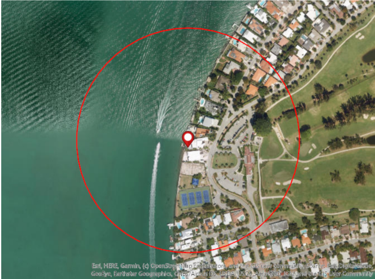
Figure 2. Image showing the action area defined by the extent of behavioral noise effects based on the proposed action’s installation of 12-inch wood piles using impact hammer (ArcGIS). The red circle delineates the radius where endangered species could be exposed to potentially harmful noise levels (705 ft).
