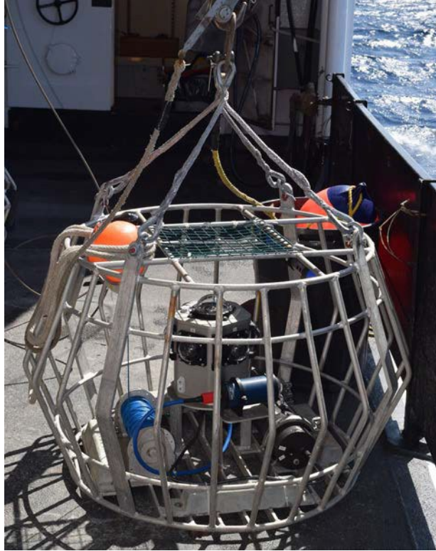
Figure 6. SatCam Array with sonde mounted, used to sample natural reefs and low relief artificial reef.
