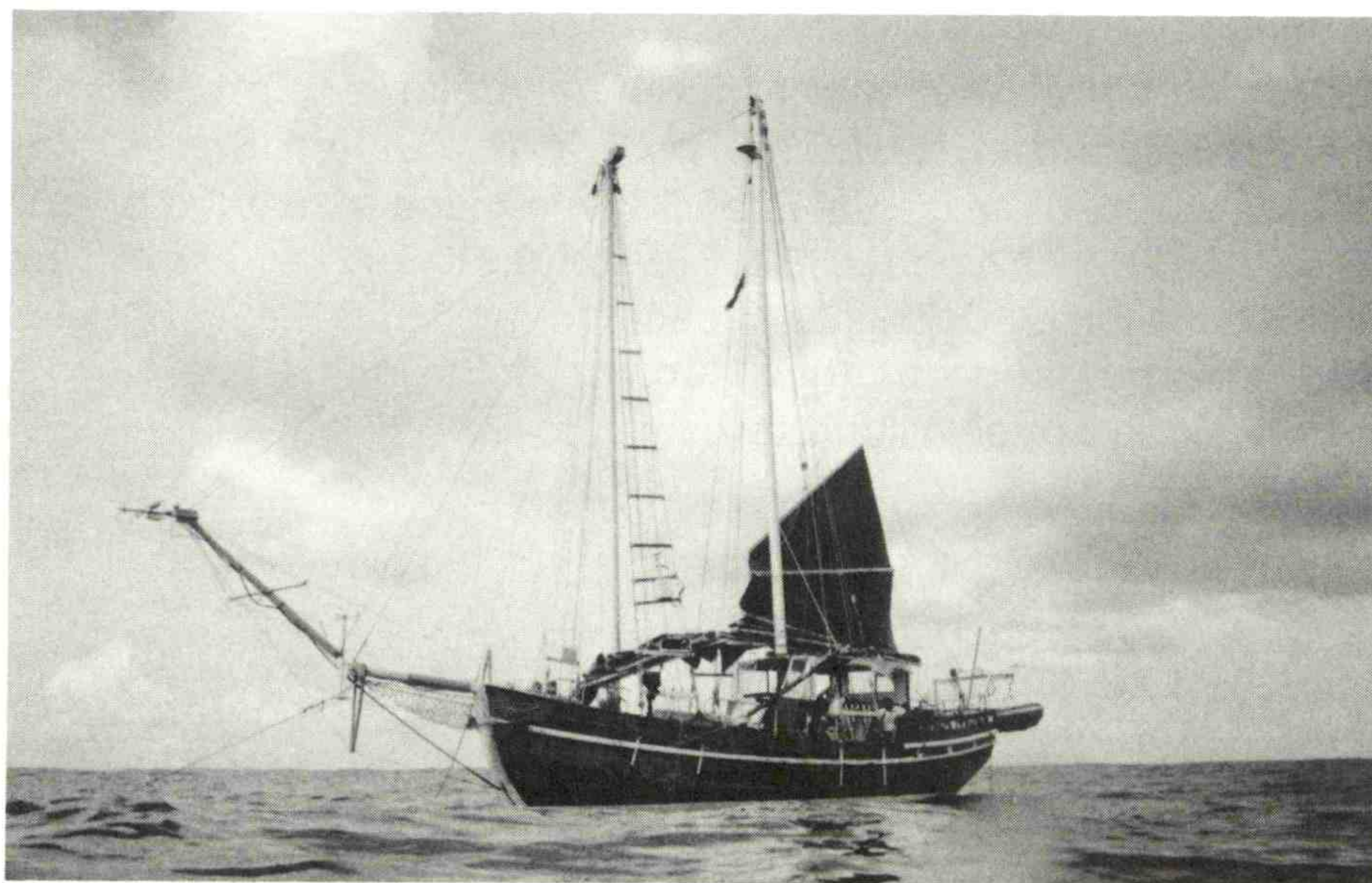
The sailing vessel Malaita was instrumented with an eddy correlation flux measurement system for determining air-sea interactions during TOGA/COARE.
