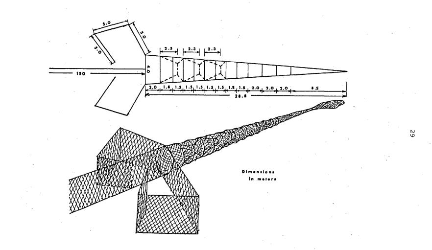
Figure 4.- Diagram of a traditional fishing device used for capturing saffron cod in Pacific waters of the U.S.S.R. (from Andreev 1962).
