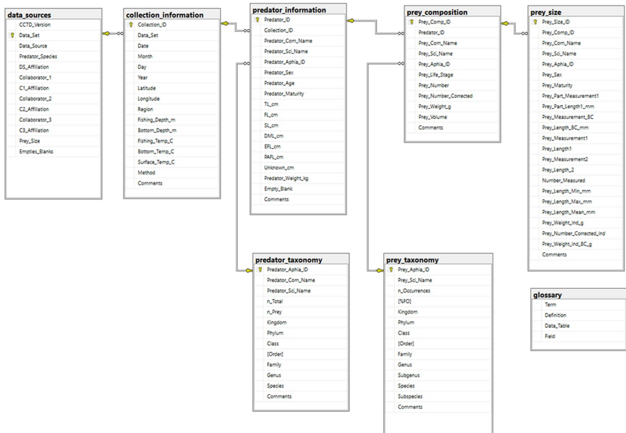
Fig. 1 California Current Trophic Database diagram. Primary keys within tables (gold keys) and foreign key relationships between tables (infinity symbols) are indicated. Primary key = a unique identifier for each row in a table. Foreign key = a set of attributes in a field of one table that refers to the primary key field of another table. Relationships are therefore hierarchical in the direction of one (primary key, parent table) to many (foreign key, child table). TL = total length, FL = fork length, SL = standard length, DML = dorsal mantle length, EFL = eye fork length, PAFL = pre-anal fin length, BC = back-calculated, Ind = individual.
