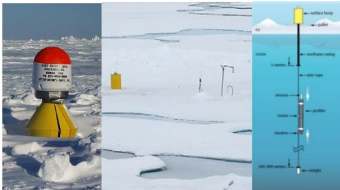
Figure 11. Example Passive Devices, Buoys (Left panel is an Ocean Flux Buoy; Center and Right panels are Ice Tethered Profilers).
