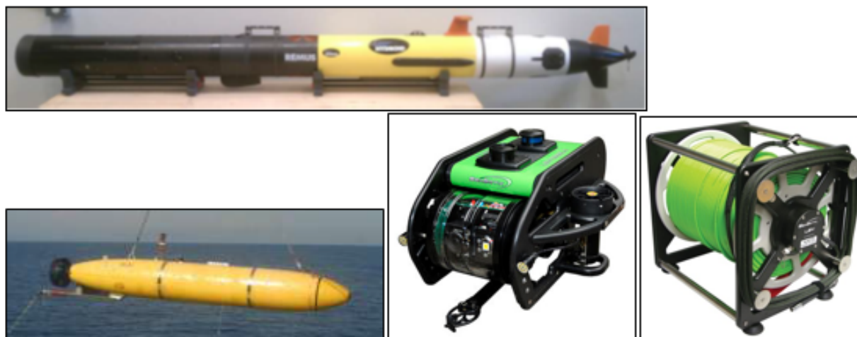
Figure 8. Examples of Unmanned Underwater Vehicles. Top panel is a Remote Environmental Monitoring Unit System 100; bottom left is a 21" Bluefin; bottom center is a Little Benthic Vehicle (LBV) 300; bottom right is the tether associated with the LBV300, resulting in a Tethered, Hovering Autonomous Underwater System.
