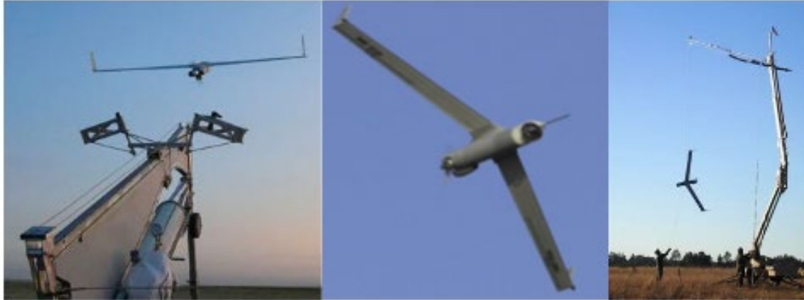
Figure 9. Example Fixed-wing Unmanned Aerial System (Left panel is launch; center panel is in flight; right panel is recovery).
