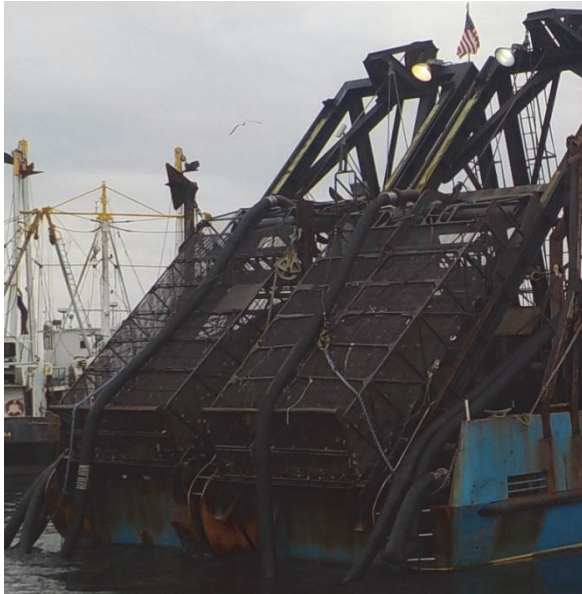
Figure 43. An example of stern-rigged dredges on A-frames.
