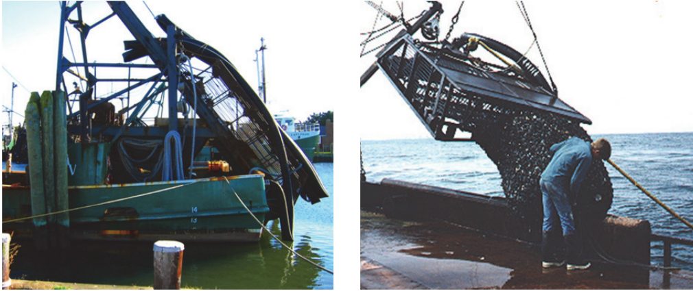
Figure 48. An example of a one-piece (left) and two-piece (right) dredge.
