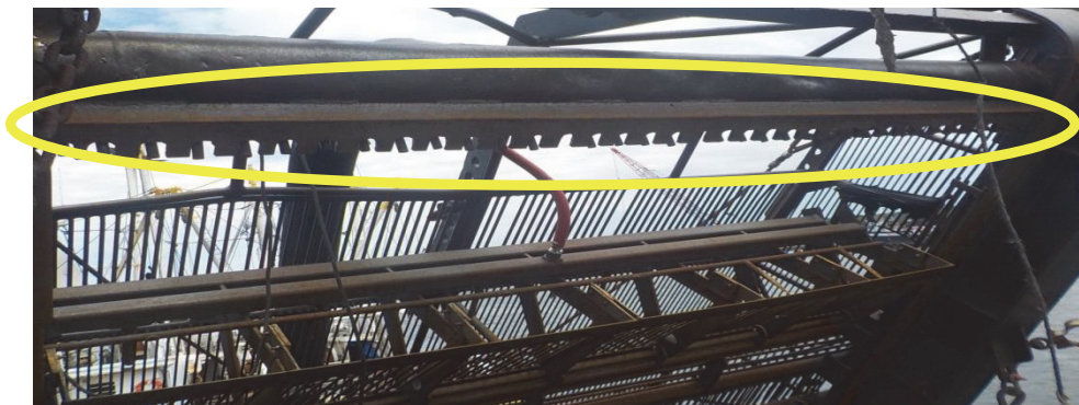
Figure 44. Example of nozzles on the manifold section of a clam/quahog dredge.
