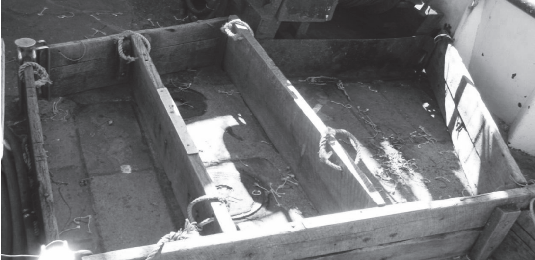
Figure 67. An example of multiple checker pen shapes present on deck. Note the ropes attached to each board, which allow the fishermen to manipulate the size and shape of the checker pen, as needed.
