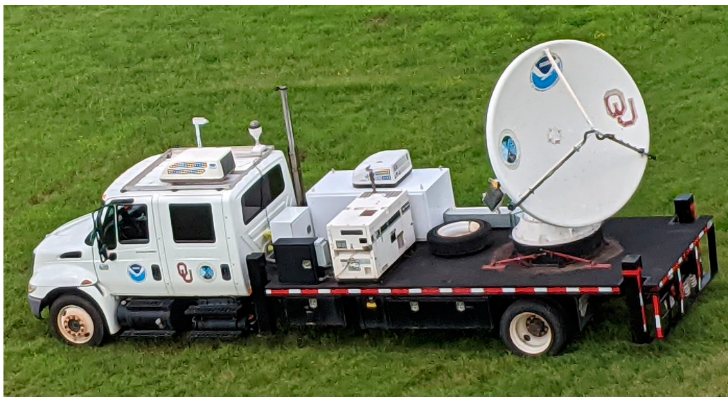
FIG. 1. The X-band mobile radar (XERES) at North Base, University of Oklahoma, in Norman.
