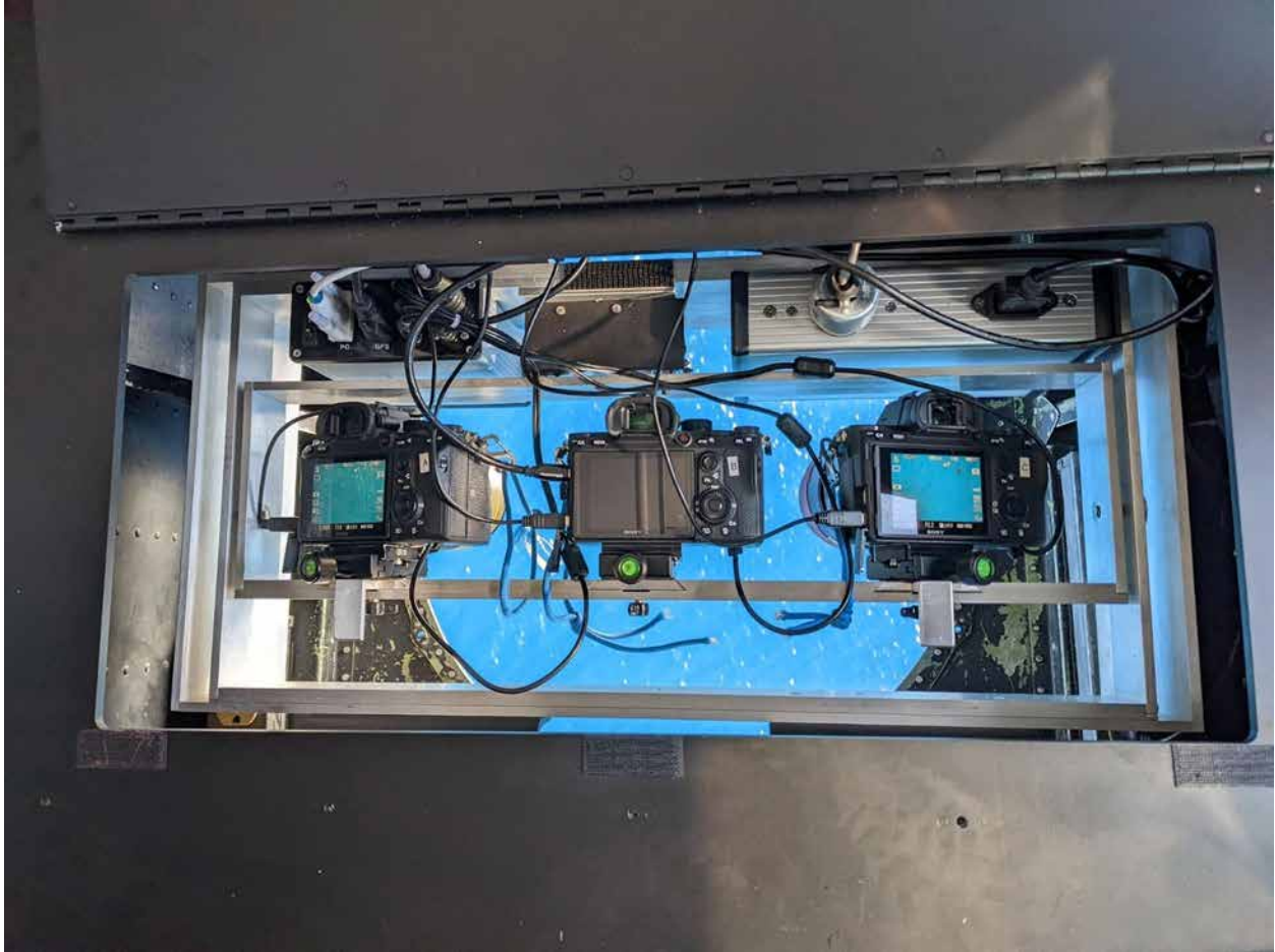
Figure 2-3 Three Sony cameras mounted on the forward motion compensated platform Platform positioned on the belly window.
