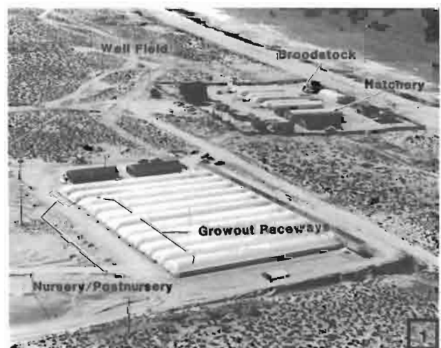
Figure 1.—Aerial view of the Universities' of Arizona and Sonora shrimp culture research facility at Puerto Peñasco. The locations of the seawater wells, the broodstock raceways, the hatchery, nursery/postnursery, and the growout raceways are indicated.
