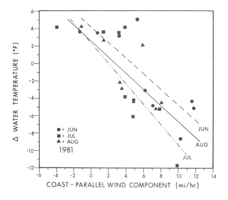
FIGURE 3. Best-fit linear regressions of water temperature change (°F) and upwelling (+)/downwelling (-) wind components (mi/hr) for high-pass filtered data ( $\triangle$  water temperatures greater than 1 standard deviation from monthly mean).
