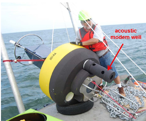
Fig. 4. Surface acoustic modem well attached to the base of the buoy hull, before acoustic modem is inserted.
