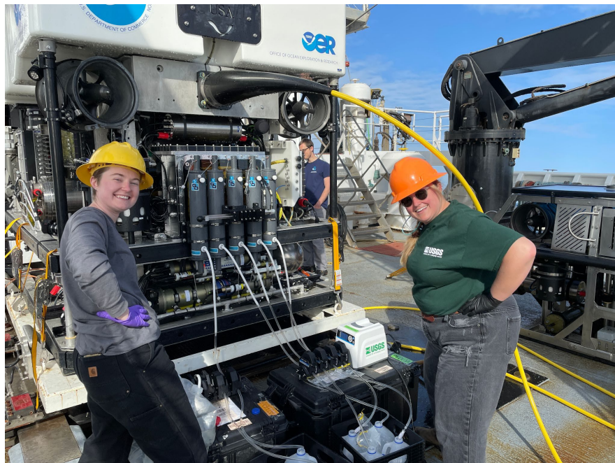
Figure 3. Science leads Paige Koenig (left) and Alexis Weinnig (right) process water samples using the USGS peristaltic pump system (lower) to extract water samples from the Niskin bottles on ROV Deep Discoverer .
