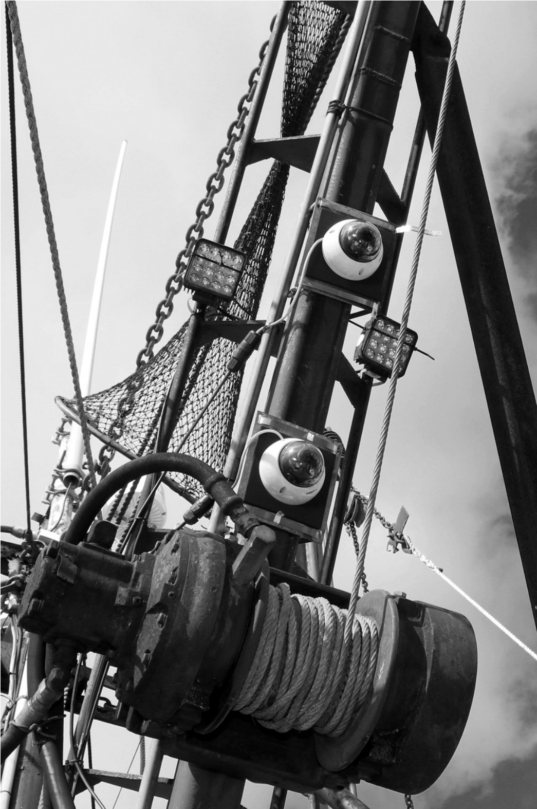
Figure 2: EM surveillance cameras mounted to a vessel's rigging (image courtesy of Gulf of Maine Research Institute)
