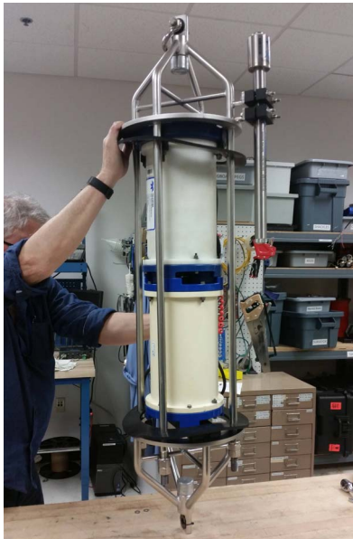
Fig. 3. ADCP, extra battery canister, and locator beacon installed in mounting cage of the 58 inch diameter ellipsoid buoy.
