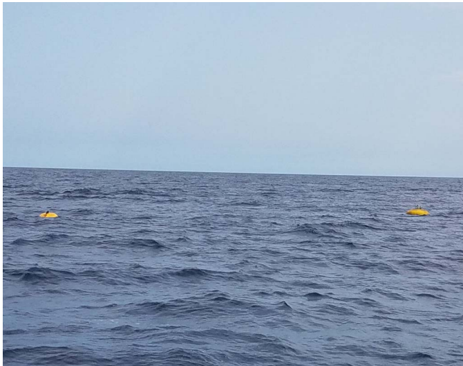
Fig. 7. Both of the mooring systems ellipsoid buoys surfaced following acoustic release from sea floor upon recovery.
