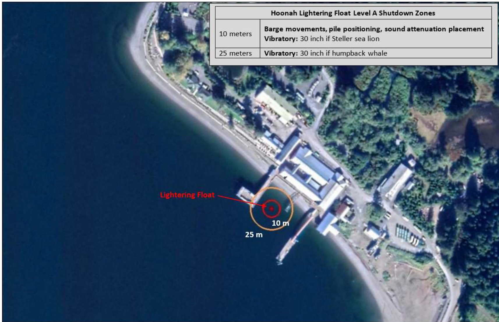
Figure 1. Level A Shutdown Zones at the Lightering Float construction site. Zones described in Table 2.
