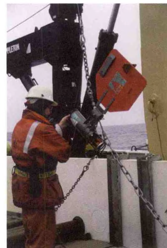
A current meter (an instrument that measures current, temperature, conductivity, and pressure) is recovered by an operations specialist aboard the R/V Miller Freeman from a sub-surface oceanographic instrumentation mooring deployed in the Bering Sea by FOCI/PMEL in support of Steller sea lion habitat studies.
