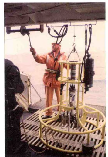
CTD array is deployed off NOAA R/V Miller Freeman to take conductivity, temperature, and depth measurements.
