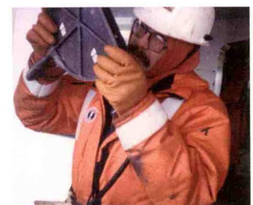
NMFS scientist measures wire angle to deploy CTD array.
