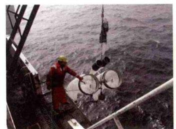
NMFS scientist deploys bongo nets with Seacat instrumentation to support studies on the growth and survival of fish larvae.
