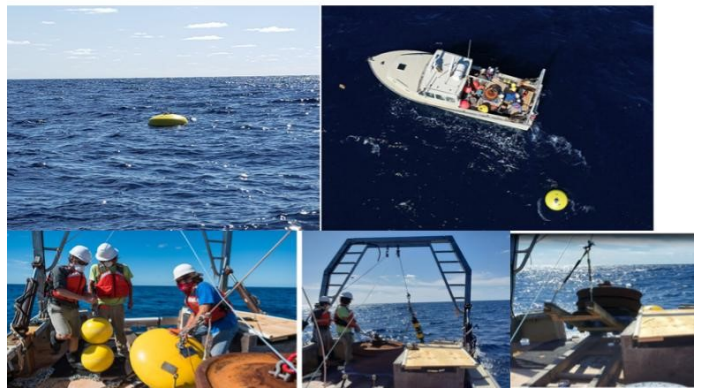
Fig. 5. Deployment photos - clockwise from top left: large elliptical buoy deployed, view of the deployment from drone footage, anchor being moved into place, tabletop for fairing installation, preparation of smaller elliptical buoy
