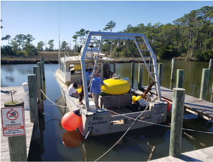
Fig. 4. RV Miss Caroline used to deploy and recover the mooring with the mooring visible on the deck
