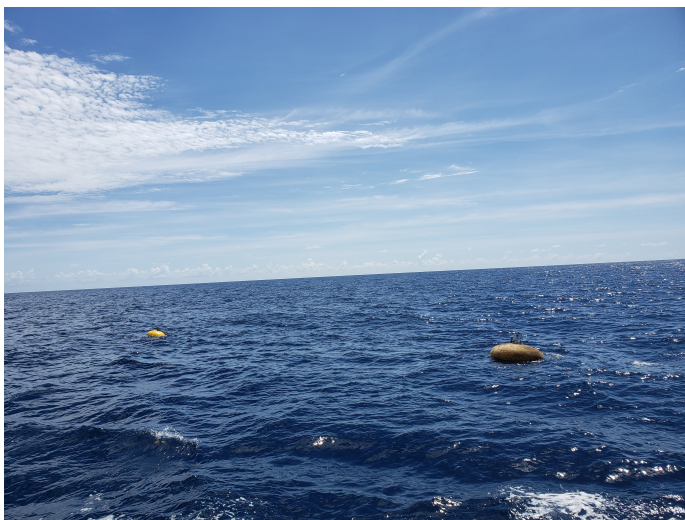
Fig. 6. Both of the mooring systems ellipsoid buoys surfaced following acoustic release from sea floor upon recovery
