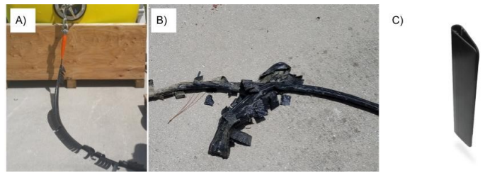
Fig. 2. A) Field test one fairings before deployment, B) Field test one fairings after deployment, C) Field test two, snap on fairing example
