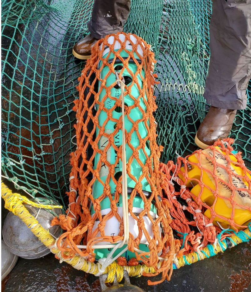
Figure 2. --SBE 19plus V2 SeaCAT Profiler CTD in a PVC housing attached behind the trawl headrope during the 2022 eastern Bering Sea survey.
