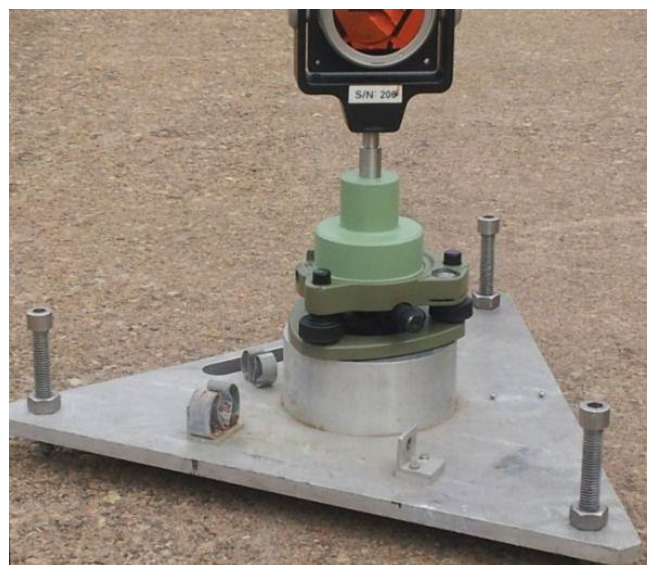
Figure 13: NGS trivet used on supplemental points
