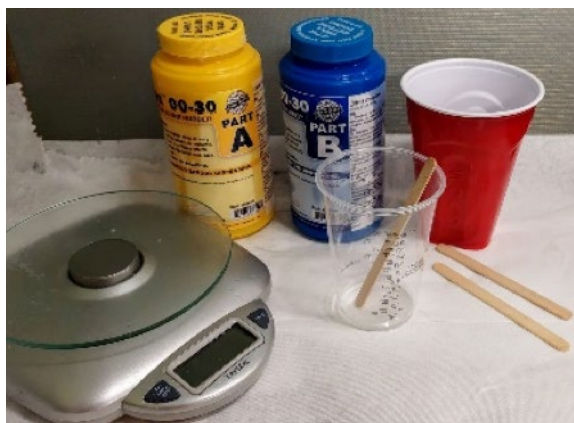
Fig. 6. Materials necessary for casting with EcoFlex silicone rubber.
