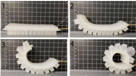
Fig. 10. Stages of pneumatic actuation for chamber network gripper prototype cast out of silicone using a custom designed, 3D printed mold.
