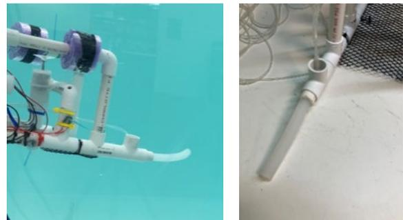
Fig. 8. PVC Pipe Gripper mounted on SeaPerch ROV.
