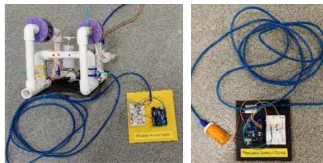
Fig. 5. SeaPerch II ROV outfitted with whisker sensors (left). Educational Demo for pressure sensor (right).
