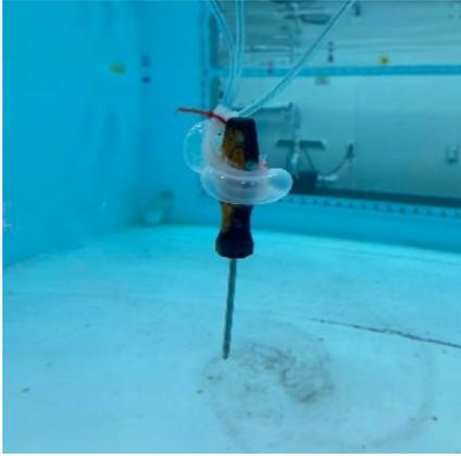
Fig. 9. A functional three-chambered pen gripper prototype successfully using hydraulic actuation to holding a screwdriver underwater.
