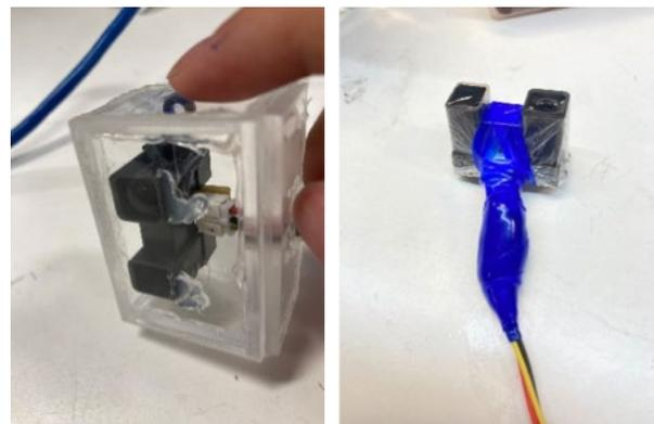
Fig. 11. Sharp IR range sensor waterproofed with acrylic box (left) and plastic wrap (right).
