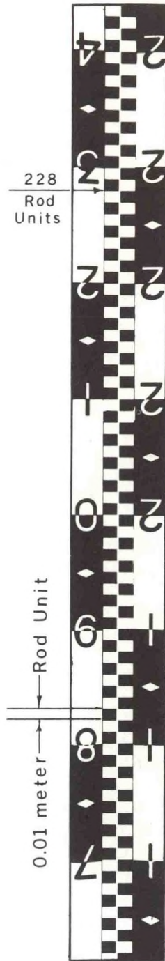
Figure 1.--Fischer Invar-scale leveling rod.
