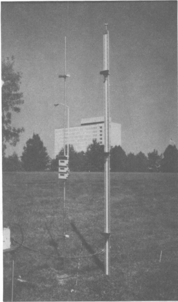
Figure 6.—Air and invar band temperature sensors.
