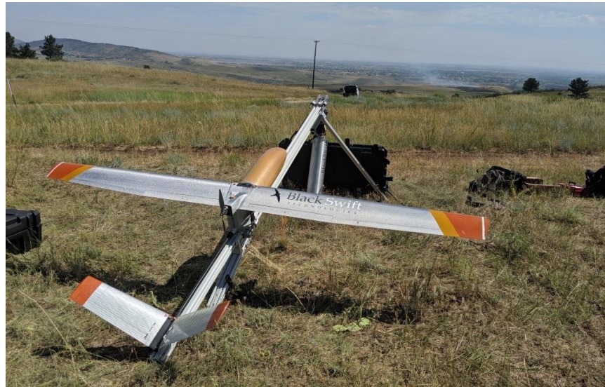
Figure 6. An S2 UAS carrying an AWSM payload ready for launch, Rabbit Mountain prescribed burn, Boulder County, Colorado, 31 July 2019.
