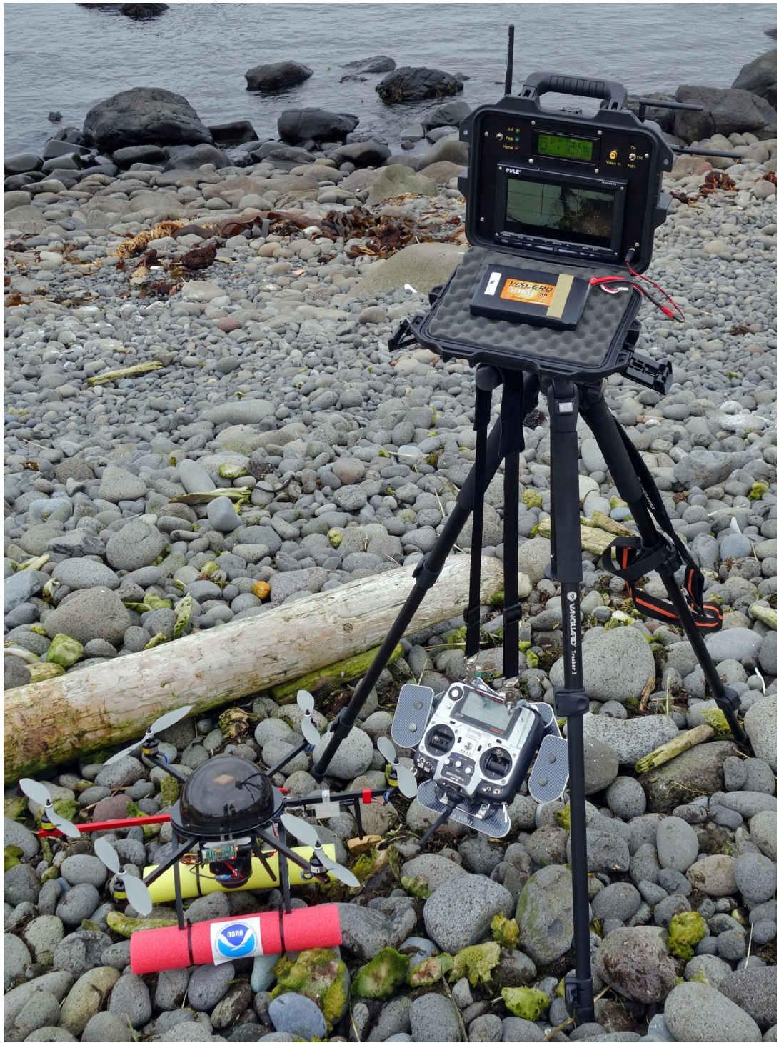
Fig. 3. The APH-22 hexacopter system including the six-rotor aircraft (left), ground station (mounted on the tripod), and the radio control transmitter (bottom, right).
