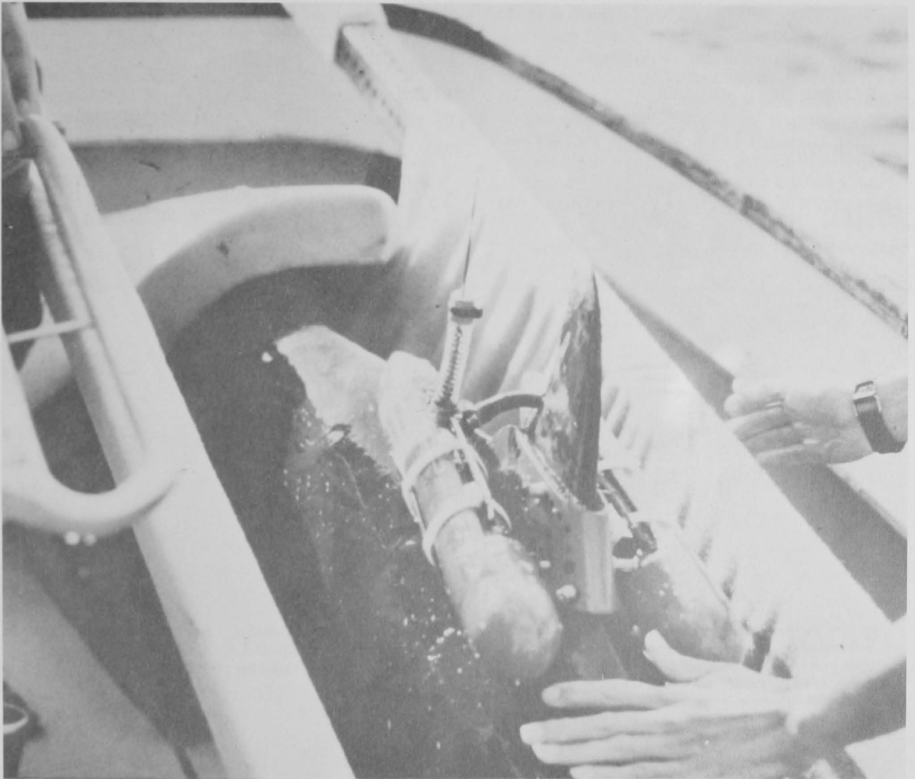
Appendix Figure A-19.—A satellite linked radiotag recently developed for attachment to small whales and dolphins. (Photo by J. Jennings, courtesy of NMFS.)
