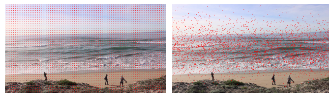
Fig. 8: Seeding strategies: We used regular grid to seed pathlines when testing. For training we used importance seeding.
