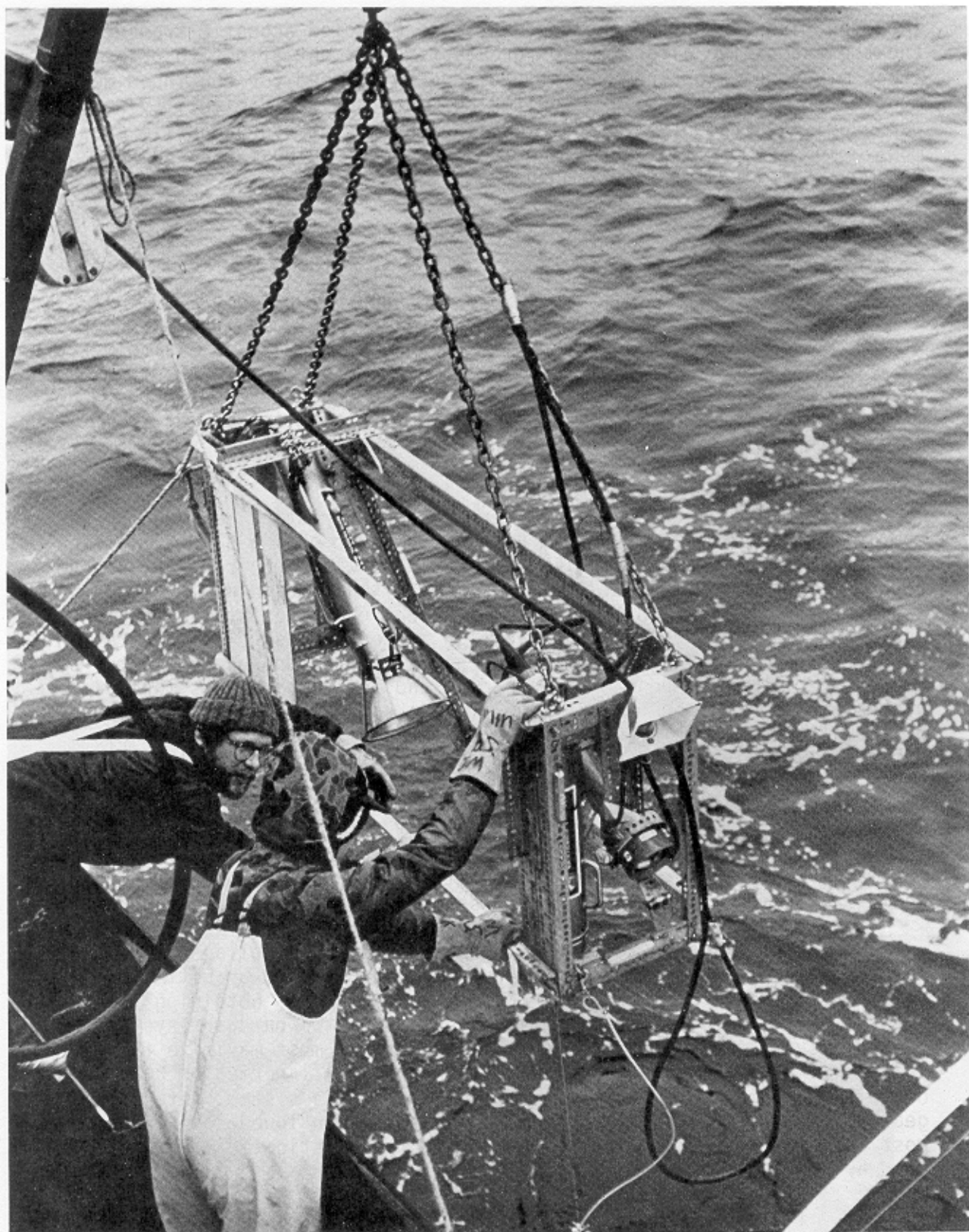
Figure 7. Camera, television and still, and light systems used in fish and invertebrate confirmations (Photo from S.C. Marine Resources Dept.).
