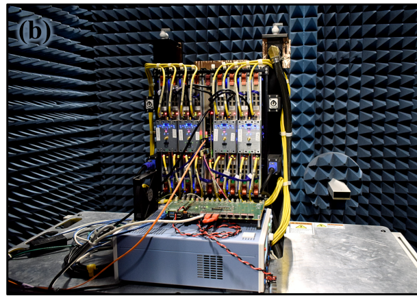
Fig. 2. Near-field scanner setup to fully characterize the H and V antenna patterns of the Horus system with (a) front (b) back view.
