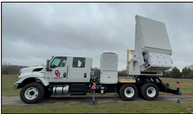
Fig. 1. Photograph of the mobile, fully digital, S-band polarimetric phased array radar called “Horus.” The system consists of 25 panels each with 8 \times 8 dual-polarization elements (1,600 polarimetric elements in total).
