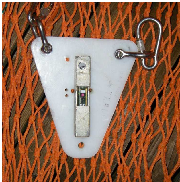
289 290 Figure 2. Archival tag affixed to polyurethane base plate assembly with shackles at the forward corners.
