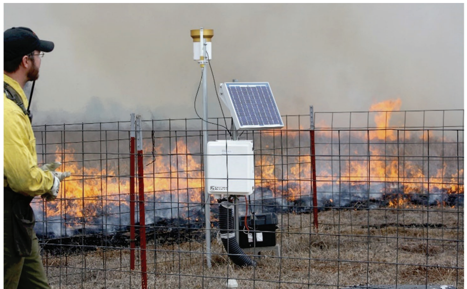
A fire manager supervises a prescribed fire near a soil moisture monitoring station in a tallgrass prairie ecosystem at the Marena, OK In Situ Sensor Testbed. Soil moisture data can help identify hazardous fuel conditions as well as optimal conditions for fuel treatment and post-fire restoration. Photo courtesy of Jeff Basara, University of Oklahoma.
