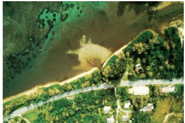
Runoff from upland areas causes excessive sedimentation that can smother near-shore coral reefs. Source: Guam CMP (credit: D. Limtiaco)
