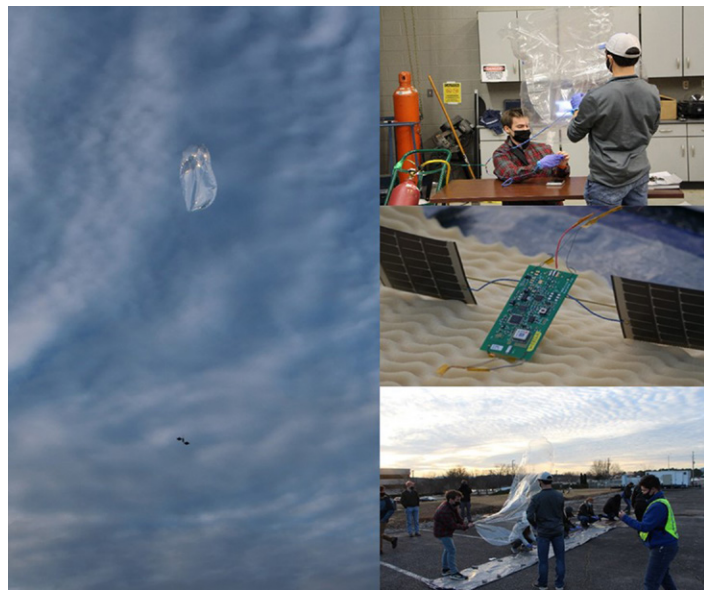
Fig. 3. (left) Superpressure balloon with SkyTracker just after launch. (top right) Members Todd McKinney and Nick Perlaky measuring lift of balloon on a gram scale. (middle right) SkyTracker payload with two 4.8-V solar panels on either side. (bottom right) Paula Tucker (yellow vest) and fellow team members prepare to launch the first balloon.
