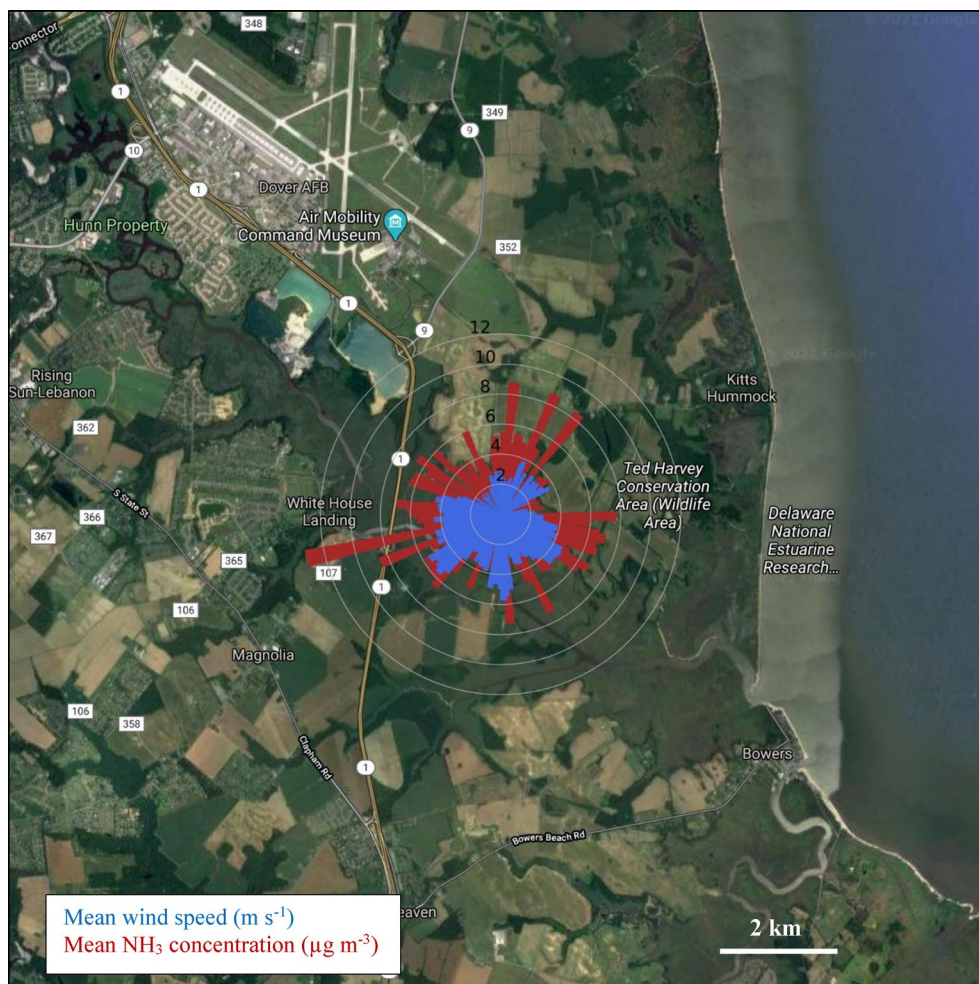
Figure 5. Wind rose derived from the data collected during the entire study period. Red wedges correspond to mean ammonia ( \text{NH}_3 ) concentration ( \mu\text{g m}^{-3} ) as a function of wind direction, and blue wedges correspond to mean wind speed ( \text{m s}^{-1} ) as a function of wind direction. The background image is a satellite view of the study site location and neighboring areas derived from Google Maps.
