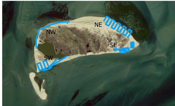
Fig. 2. Tracks of APH-22 flights performed for multi-stage image collection in Muskeget Island quadrants (NW, NE, SE, and SW).
