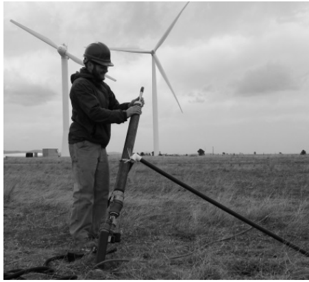
Figure 4: Air cannon is used to launch tennis balls to mimic bird impacts at NREL-NWTC.
