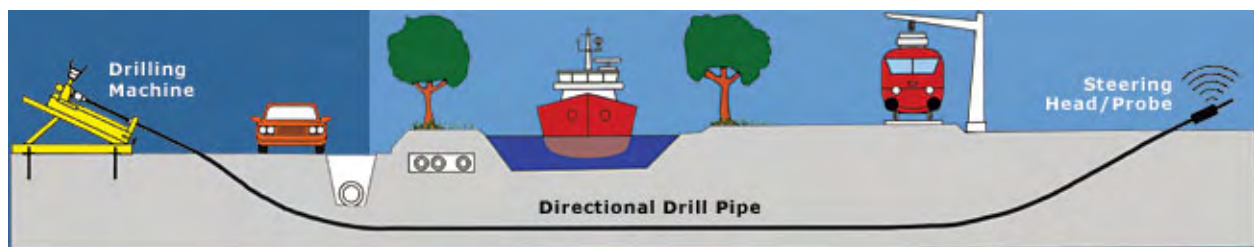
Horizontal Directional Drilling Illustration. Source: http://www.perforator.net/hdd.html
