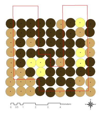
**Figure 8(C).** Mean bottom slope was calculated for each bathymetric grid cell in the study area. The absolute values of these slopes were then averaged within the 400-m detection range for each station. The lighter values represent small slopes (flat) and darker areas represent larger slopes.
