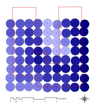
**Figure 8(B)**. Three sediment classifications were generated based on sediment grain size values calculated from ground-truth reflectance values from sidescan sonar data. These values were averaged within a 400-m receiver detection range and displayed with a corresponding sediment classification. Light yellow represents coarse grain sizes, light brown is intermediate and dark brown represents fine grain sizes.
