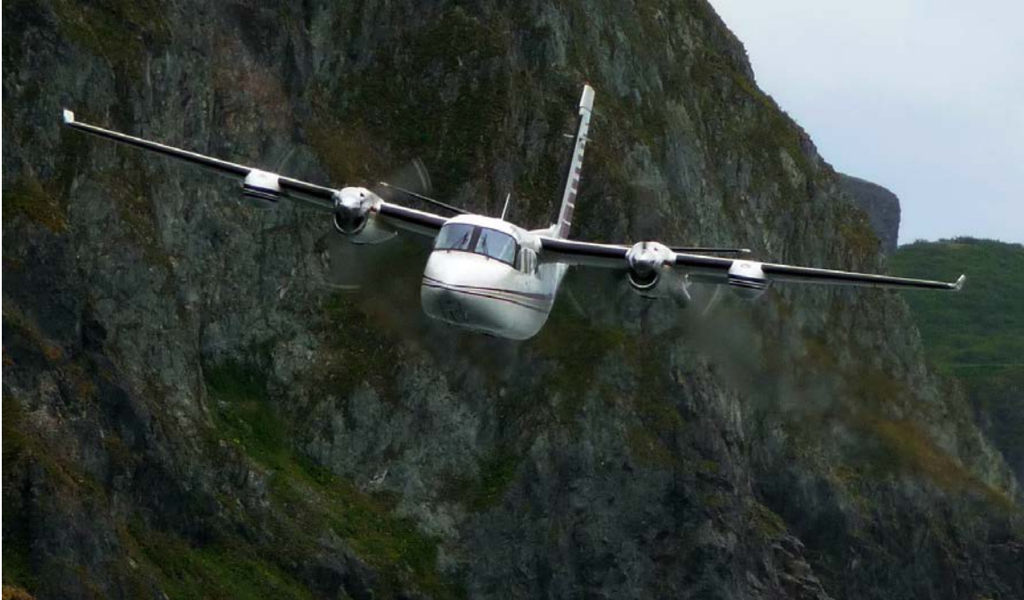
Figure 2. --Twin engine, high wing Aero Commander 690 survey platform used during Cook Inlet beluga whale aerial surveys, June 2014 (photo courtesy of Clearwater Air, Inc.).
