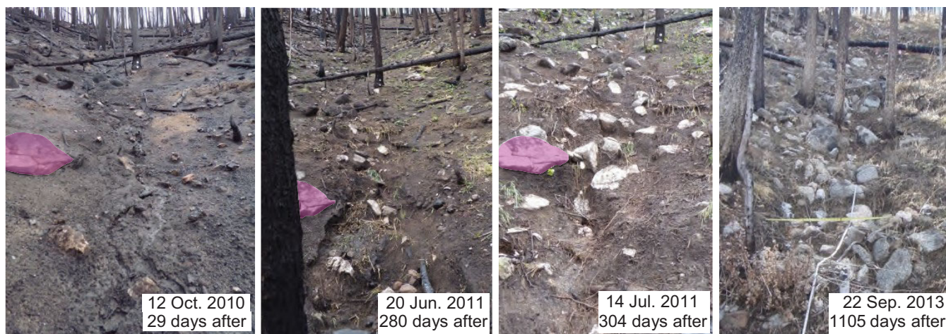
Figure 12. Time series of photographs near the headwater catchment outlet where the surface runoff flume was located prior to removal. The pink shaded rocks mark common points between the photographs for comparison of changes in channel morphology and the emergence of cobbles and boulders. The 2013 photograph was taken by J. Moody.
