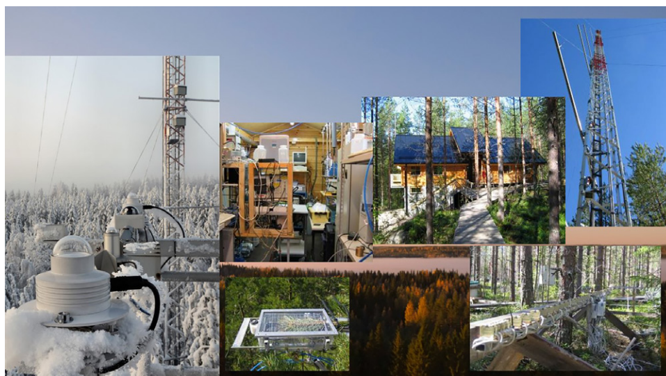
Fig. 1. Elements of the boreal forest station Hyttiälä in Finland that measures the controlling variables in this ecosystem. It is an example of a comprehensive global Earth observatory (Kulmala 2018). As in other ICOS and ACTRIS stations across Europe, measurements cover variables in the atmosphere, biosphere, soil, and lake, which characterize water and energy flow and exchange, atmospheric chemistry, micrometeorology and cloud microphysics, water and nutrient content of soil and gas exchange with the atmosphere and the biosphere, and other processes. The observatory supports several platforms (some of these outdoor and laboratory instruments are illustrated).
