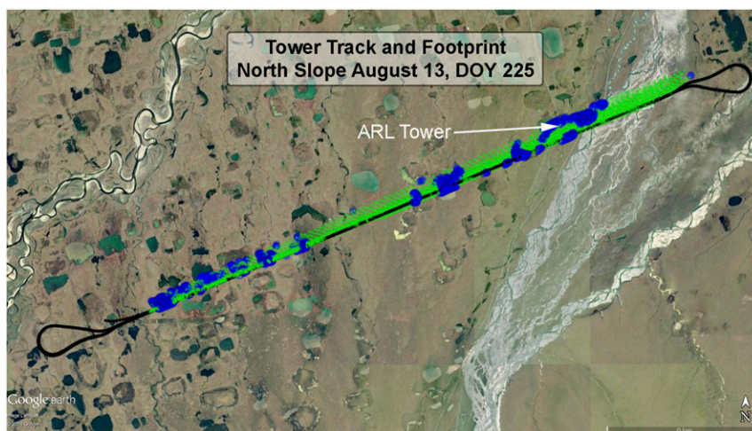
FIG. 2. Flight track past fixed surface tower with footprint spots from 13 Aug 2013 showing water (blue spots) and other surface types (green spots), of which wet sedge has the largest fraction and the strongest \text{CH}_4 emission. Prudhoe Bay is 20 km north of the ARL tower.
