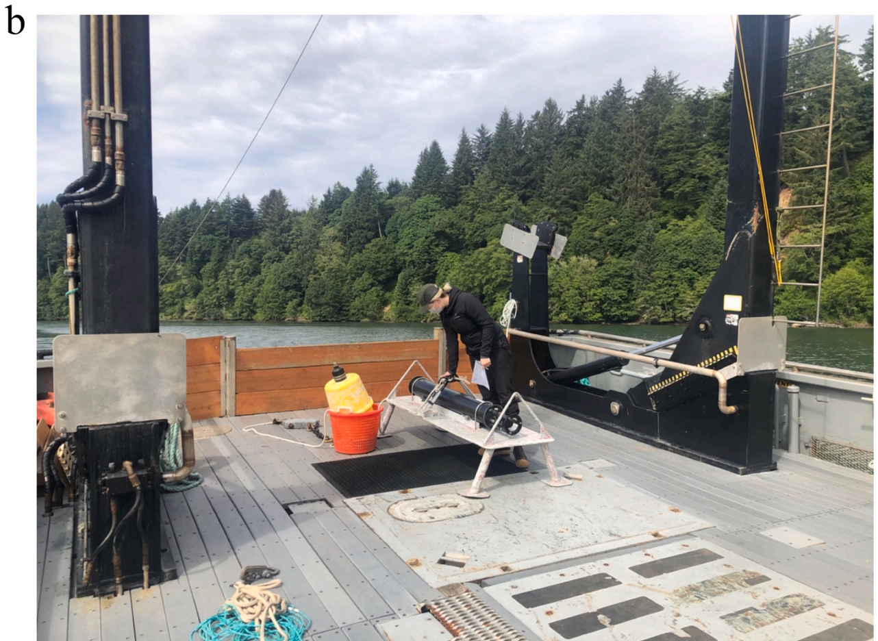
Fig. 2. a. Mooring diagram showing hydrophone and acoustic release. b. Scientist L. Roche prepares the hydrophone (mounted on metal lander) and attached acoustic release (yellow buoy) for deployment near Newport, OR. (For interpretation of the references to color in this figure legend, the reader is referred to the web version of this article.)
