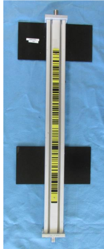
Figure E-1. Sighting target with invar strip attached.
