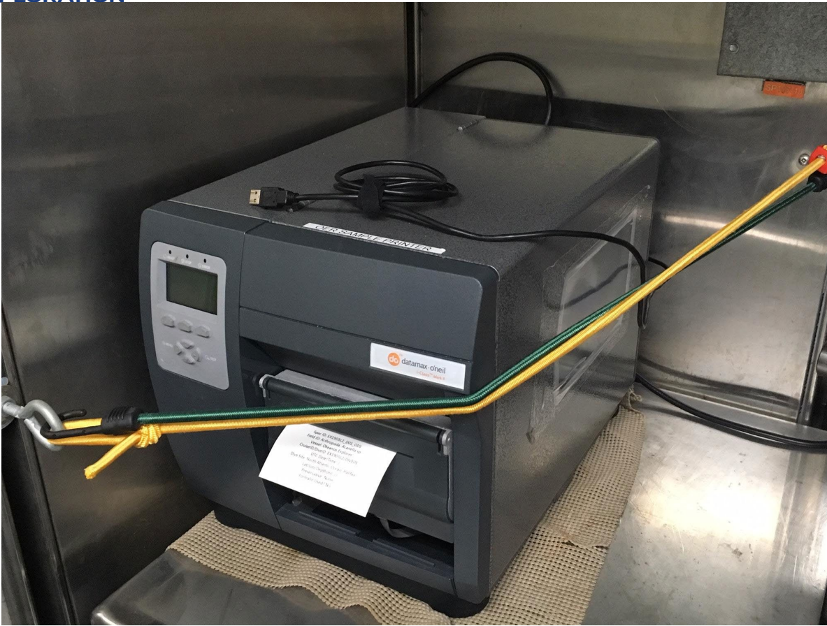
Fig 13. The Datamax O'Neil label printer in the port corner of the wet lab. The printer cable needs to be connected to the back of the Sample Data Management laptop for label printing.
