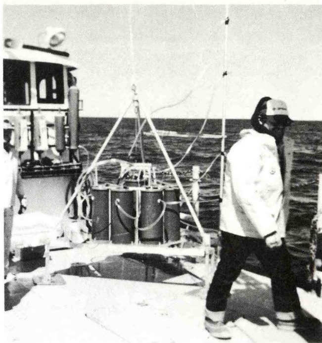
Deployment of a water sampler tripod for a near-bottom experiment. One important function of the RV Shenehon is the deployment and retrieval of the instruments used to collect basic data.
